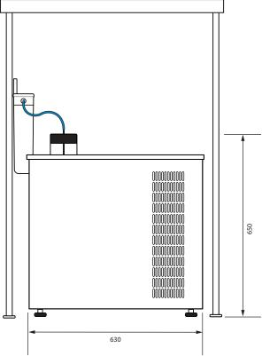
N.B. When trimming tubes to length - to ensure NO LEAKS use a sharp tube cutter for a clean cut ALL DIMENSIONS GIVEN ARE IN MM.
