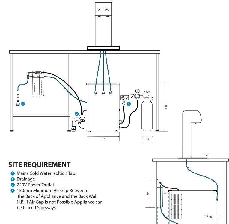
**Please Note:** If the appliance is installed in a closed cupboard space, large adequate ventilation is required to validate the warranty
