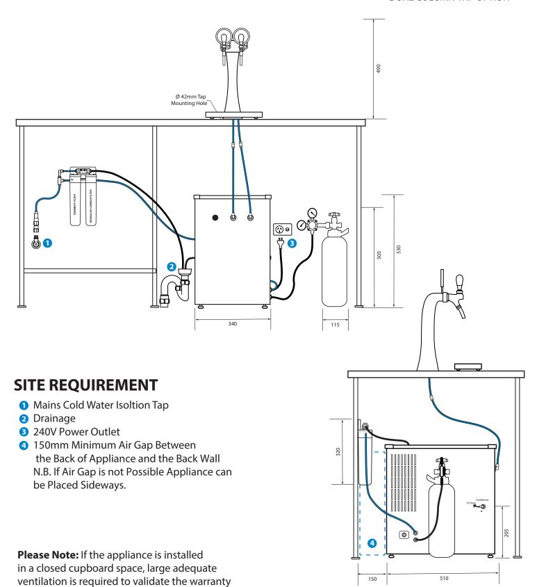
N.B. When trimming tubes to length - to ensure NO LEAKS use a sharp tube cutter for a clean cut
